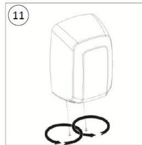
Screw the cover fixing screws (x2) Your dryer is now ready to be used on a Plug-in base
